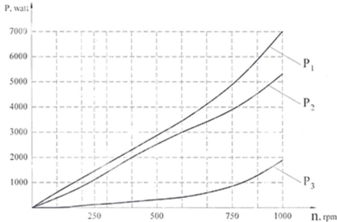
Fig. 3. Dependencies of the power  $P_1$  required to drive a brush drum,  $P_2$  to overcome the resistance of air to the rotation of brush and  $P_3$  to combing of leaves and seeds of alfalfa from the rotation speed  $n$  of the brush drum
