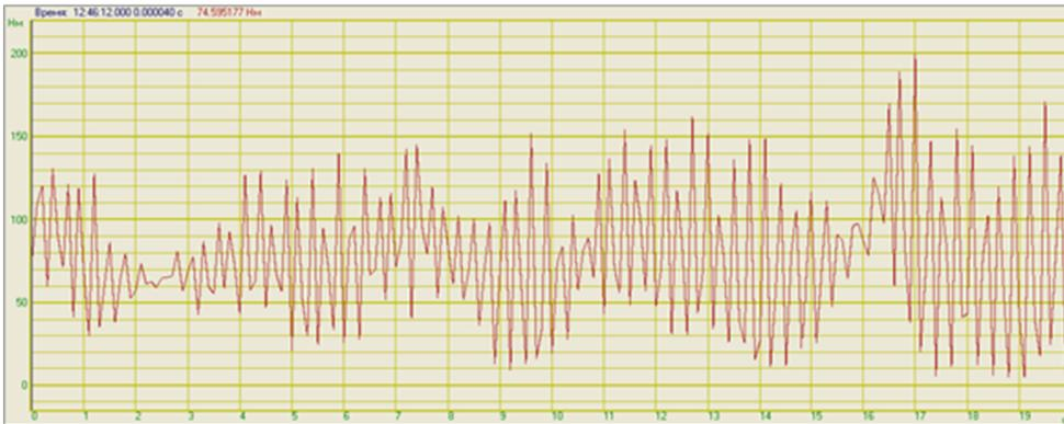
Fig. 5. Oscillogram of the sweep of the stripping device universal machine for harvesting alfalfa seeds and stamping
